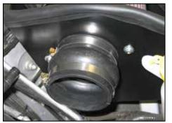
20. Install the provided hump hose (084057) onto to the filter adapter and secure with the provided hose clamp.
