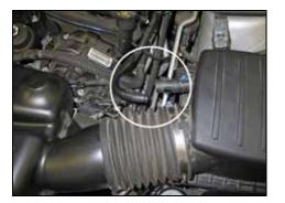
4. Disconnect the crank case vent tube from the air box as shown.
