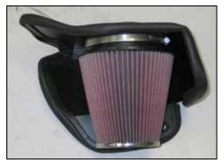
15. Install the K&N<sup>®</sup> air filter onto the filter adapter and secure with the provided hose clamp. NOTE: Drycharger<sup>®</sup> air filter wrap; part # RF-1041DK is available to purchase separately. To learn more about Drycharger<sup>®</sup> filter wraps or look up color availability please visit http://www.knfilters.com<sup>®</sup>.
