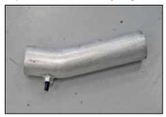
18. Install the inlet air temperature sensor into the  $K\&N^{\ensuremath{\mathbb{R}}}$  intake tube as shown.
