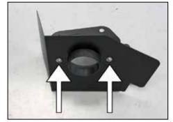
11. Install the filter adapter into the heat shield and secure with the provided hardware.
