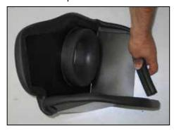
12. Install the provided edge trim onto the heat shield as shown. **NOTE: Some trimming of the edge trim will be**
