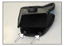
14. Install the two air box mounting grommets into the heat shield as shown.
