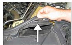
2. Lift up the engine cover to unhook it from the mounting grommets and then remove the engine cover from the engine.
