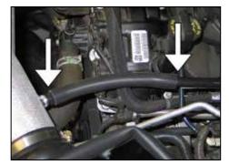
26. Install the provided crank case vent hose onto the vent fitting attached to the  $K\&N^{\oplus}$  intake tube. Connect the open end of the crank case vent tube to the factory crank case vent tube that was cut in the previous step.
