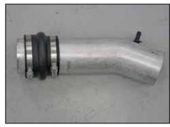
22. Slide the provided silicone hump hose (5-576) all the way onto the K&N<sup>®</sup> intake tube #27446 as shown.
